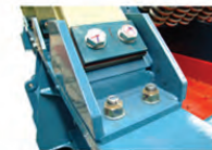
Composite slat springs maintain directional vibration control
