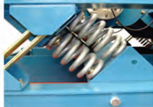
Reactor springs - designed for infinite life
